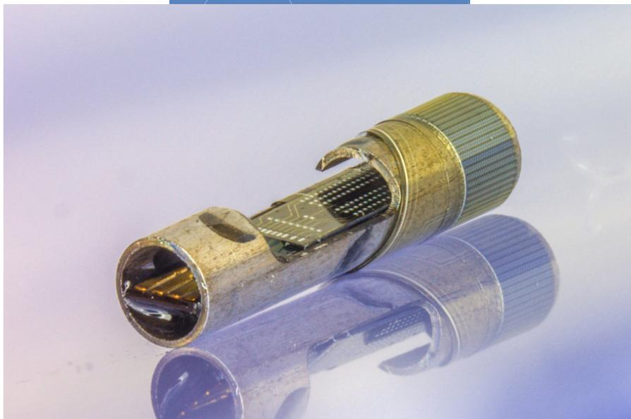
*The INCITE tip is 1.2 mm wide, and about 5 mm long. It has 96 ultra-sound transducers (compared to 64 in the previous generation technology) working at higher frequency, resulting with better resolution images.*
